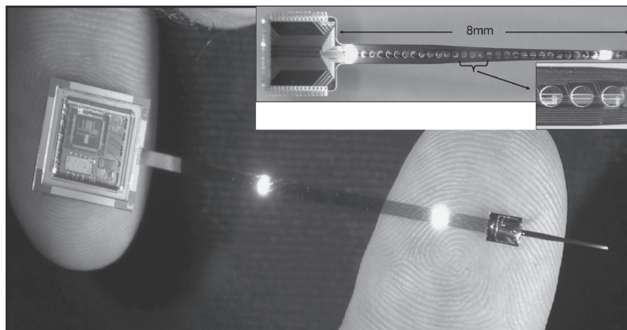
Figure 2.6. The WIMS-ERC cochlear prosthesis. (inset) The 32-site high density electrode array [32] (© 2006 IEEE).
